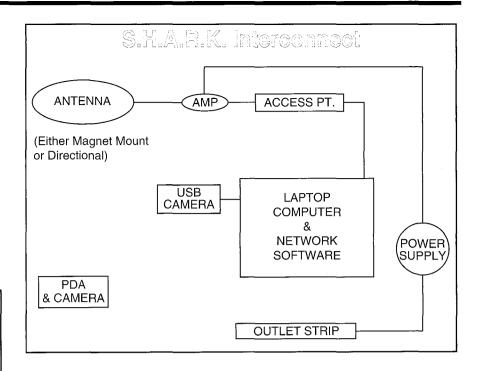
Next point the antenna to the HSMM radio repeater at the Emergency Operating Center. Ranges from several miles to 20 miles and more over open water are readily possible. Date rates can be as high as 11 million bits per second (Mbps). The actual throughput is less, because the system is operating in half-duplex mode. This is *radio*, not your local cable modem, so the radios must stop transmitting between packet clusters to listen from time to time.
